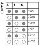
\*This is the time period the lamp remains at 100% after no motion is detected
