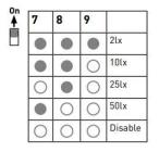
When set to *Disable*, the daylight sensor will switch the lamp on when motion is detected regardless of the ambient light level
