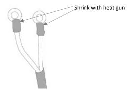
Remove the 2 screws from the Live and Neutral terminals, and ensuring correct polarity is observed, terminate Live (brown) Neutral (blue) to the screw terminals (see Fig. 5)
