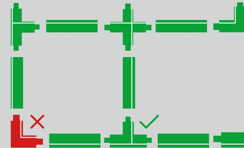
Polarity is simple with K-Line: match the L/R arrows on the connector to the track's polarity line, using the raised edge as a visual and tactile guide - ensuring safe alignment and opening the door to endless lighting configurations
