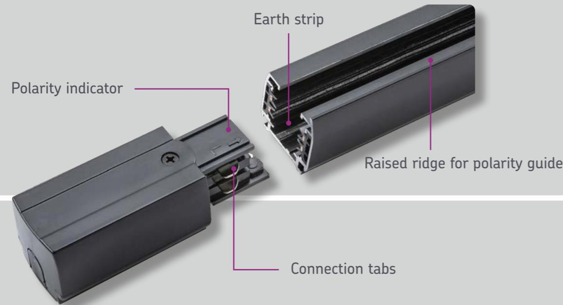
With K-Line, polarity is straightforward by design. All connectors are clearly marked with arrows and labelled "L" and "R" for left and right orientation, to be matched up with the polarity line on the track. The track itself also features a raised edge that signifies the polarity ridge - providing a simple visual and tactile guide to ensure correct alignment every time. This makes installation quicker, more intuitive, and reduces the chance of error.
